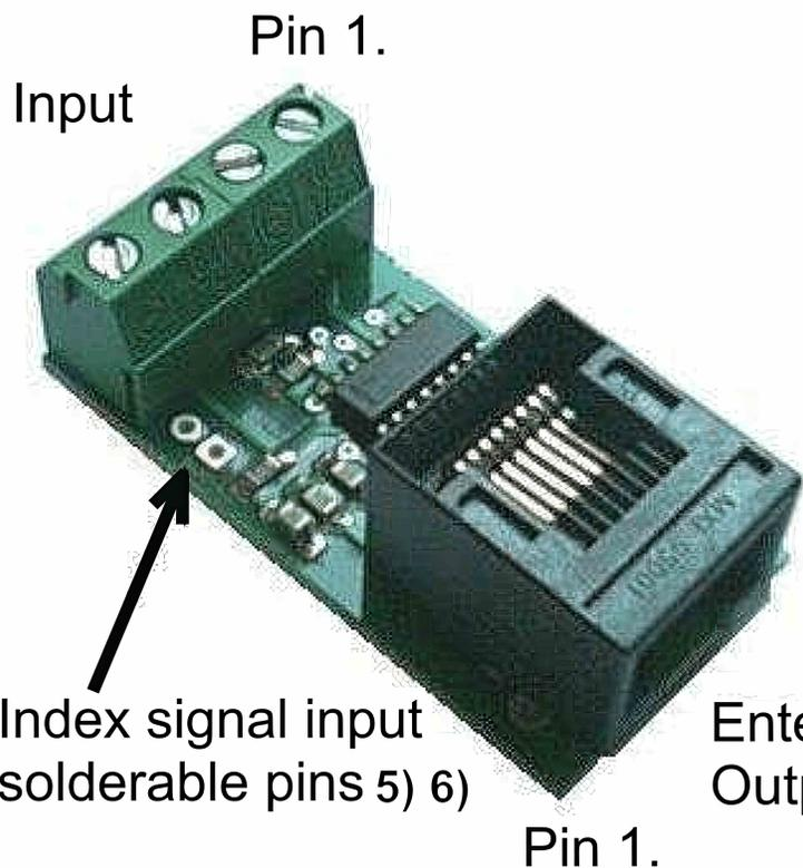
Input side pinout:
